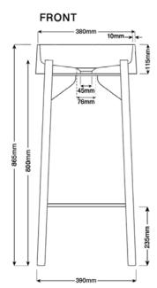
Material: Concrete + Galvanised Steel Freestanding Suits standard 32-40mm 2-piece waste, no overflow
