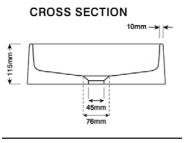
Material: Concrete Mount Surface mount Suits standard 32-40mm 2-piece waste, no overflow
