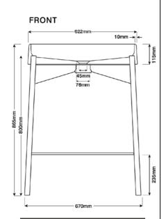
Material: Concrete + Galvanised Steel Freestanding Suits standard 32-40mm 2-piece waste, no overflow
