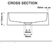
Mount Wall hung, bracket included Suits standard 32-40mm 2-piece waste, no overflow
